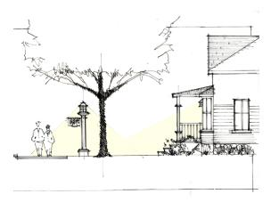
A section through the front yard of a commercial building shows how porch lights and poles can light sidewalks.
